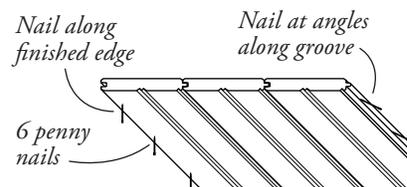
Don't forget to stagger joints!
