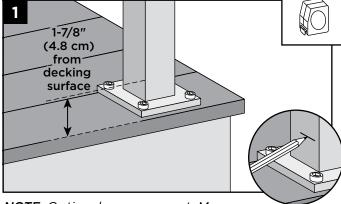
NOTE: Optional measurement: Measure 1-3/8" (3.5 cm) from top of post base plate.
